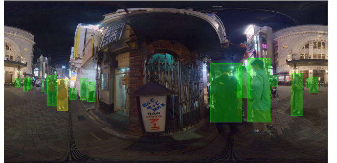
Fig. 4: The vision detection pipeline. YOLO detections are in green, and the top-1 CLIP ranking is in yellow.
